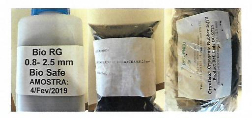
Identification: Portuguese tyre recycler; Tested ELT granulates; Particle size interval; Grinding technology
