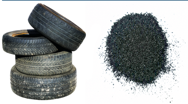
Crumb rubber (right) derived from scrap tires can be mixed into asphalt binder to improve its performance. Credit: xpixel/Shutterstock/Md Tareq Rahman.
